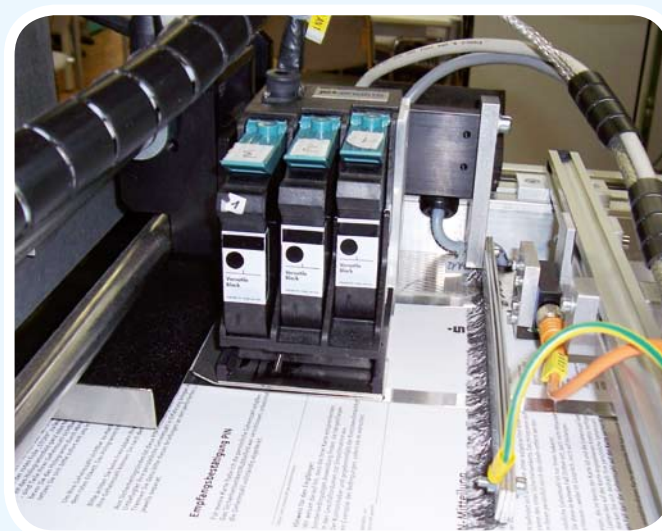
Ink jet systems are used for secure printing of PINs.
